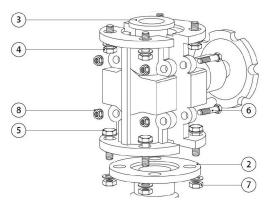
(6) and pull the valve open. Remove and replace the old rubber pipe. Reassemble SGV valve and blast machine in reverse order.
