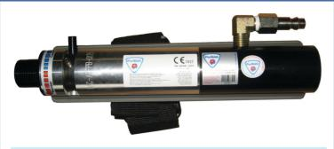
Compressed air is simply fed to the inlet, and then exits the unit either cooled or heated, depending on the setting. A simple sliding lever arrangement is provided to switch the unit between cooling and heating, and an adjustable belt for attaching Climate Controller to the operators waist, as well as protective heat shield, are each unit.
