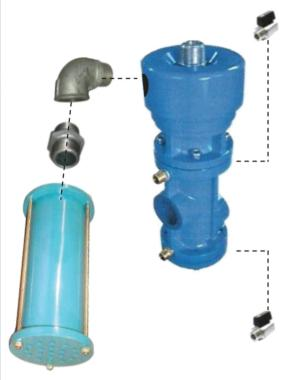
Pneumatically operated remote control system. To be used when the length of the blasting hose does not exceed 20 meters, as otherwise the delay from releasing the "deadman handle" until the closing of the air valve will be too long.
