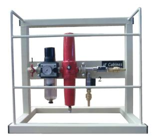
Breathing air filter on base, dual cartridges (filter / oil separation and activated carbon).
