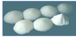
**Shoot peening:** The microbeads allow it, due to the sphericity, the available range, the hardness and the uniformity of the beads, and especially because there is no contamination of the treated surfaces to be feared. Whether it is to increase fatigue strength, or to reduce stress corrosion, prestressing is essentially a uniform hammering operation.
